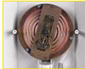
The attachment of the precision mechanism to a sturdy metal support and the extra-large pressure membrane ensure reliable zero-positioning of the pointer.
